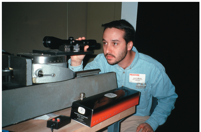
Optical quality was tested with a collimator fixture. The Redfields compared favorably with several other high-end, name-brand scopes in clarity and resolution.
