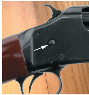
The Model 97 features shell release buttons (above l., arrows) that are pressed together to release shells from the magazine. Also, a slide-action release button (above r., arrow) is located on the right of the receiver. It allows the user to retract the slide and empty the chamber.
